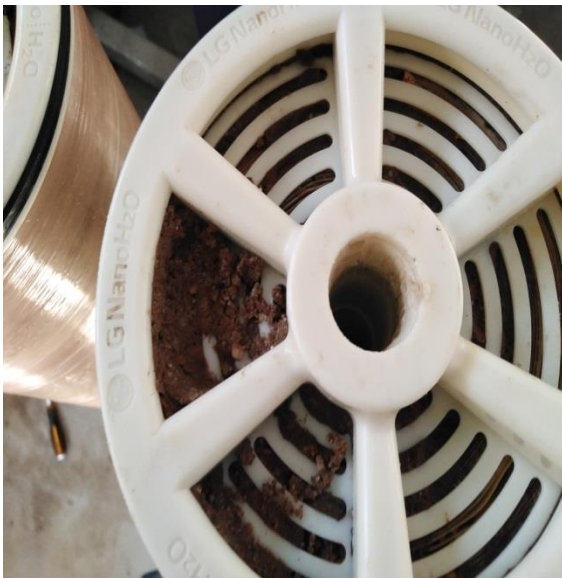
Scaling fouling Membrane
