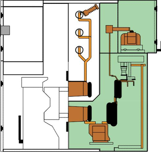
**Cable connection and VTs compartment**
