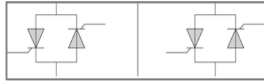
Figure 5: Thyristor topology of a “2-phase softstarter”: 2 sets of anti-parallel thyristors.
