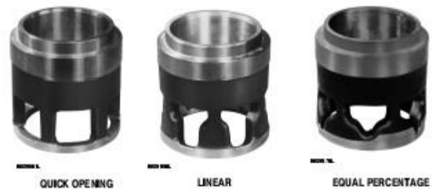
Figure 1-8. Characterized Cages for Globe-Style Valve Bodies
