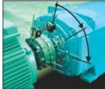
The EASY-TURN™ Program requires only 40° of rotation for an alignment solution.
