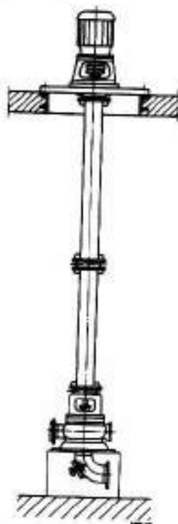
Fig. 3 Dry installation with intermediate pipe
