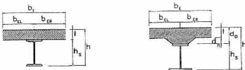
Figure 12.1 Typical Cross-Sections of Composite Beams
