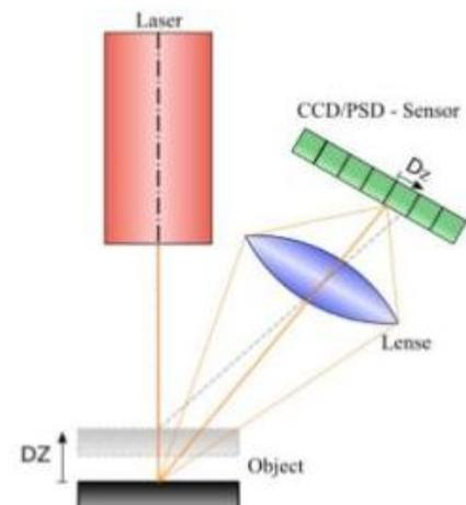
Fig -2: Laser sensor working.
