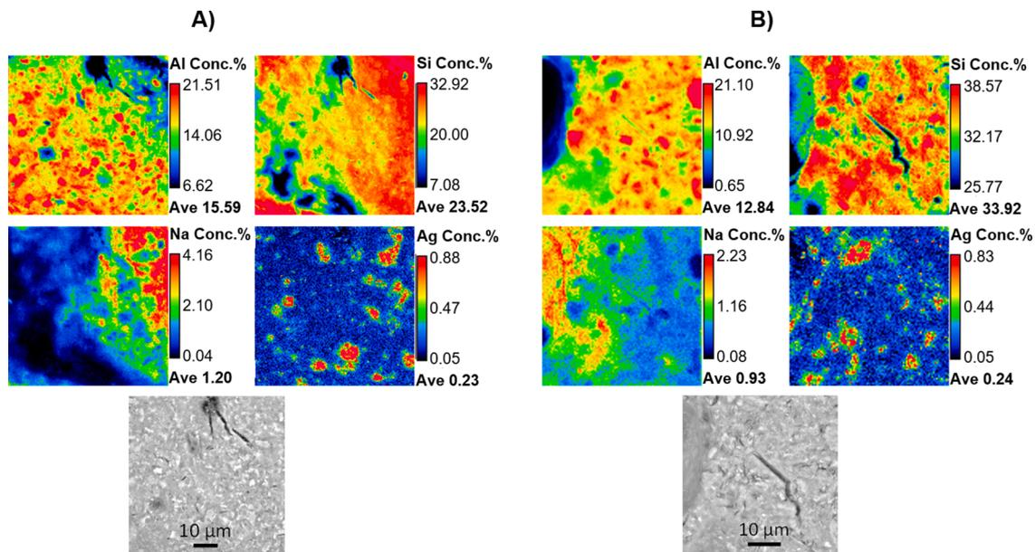
Fig. 2. Elemental maps of geopolymer foams after A) acid-flushing and B) the 3-week experiment.
