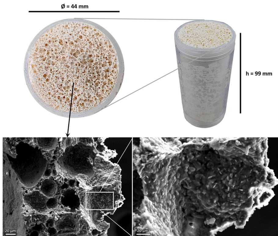
Fig. 3. Photographs and micrographs of geopolymer-bentonite composite foam.
