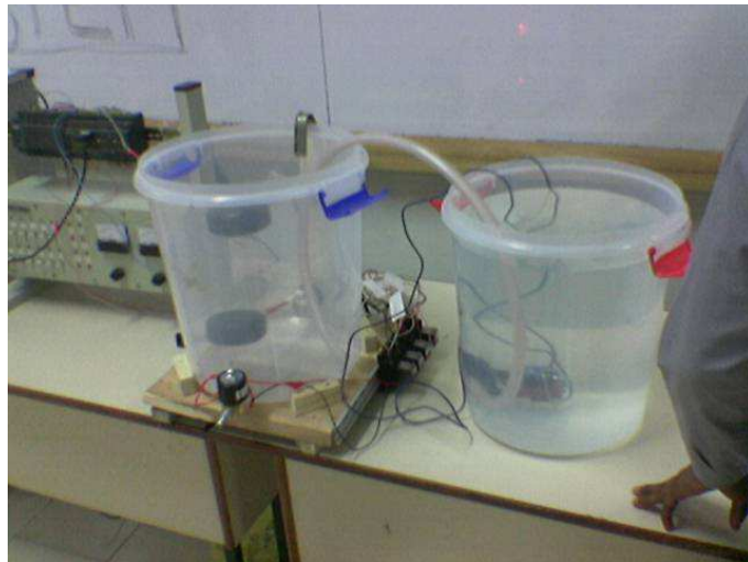
Fig 4: Water level control
