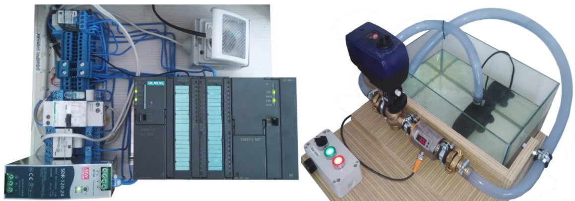
Figure 2. SIEMENS PLC configuration and the experimental stand
