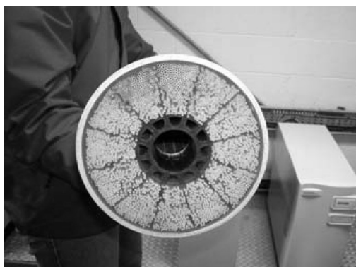
Fig. 7.7 Example of a hollow fibre membrane used in potable water treatment.
