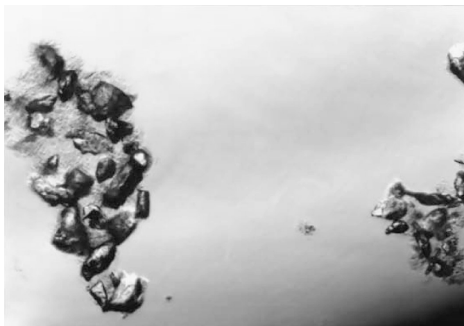
Fig. 4.9 Photograph of a ballasted floc (with kind permission of OTV – Veolia Water Systems).
