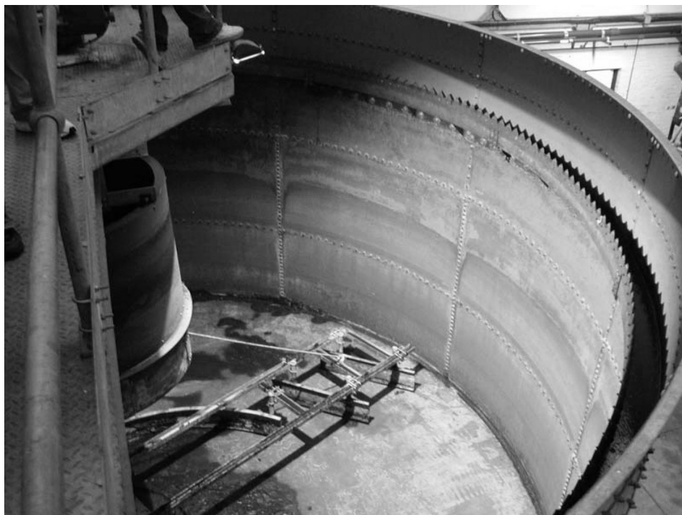
Fig. 12.4 Schematic and an internal view of a continuous sludge thickener.
